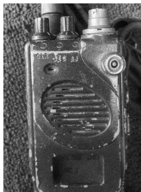
Close-up view of the Tadiran RT-7106 (PRC-710) control panel, showing selector knobs for CLR/SEC/AJ (Clear, Secure, Anti-Jamming) communication modes and an intact display window. The markings and wear indicate active operational deployment and prolonged field handling. Confidential source
