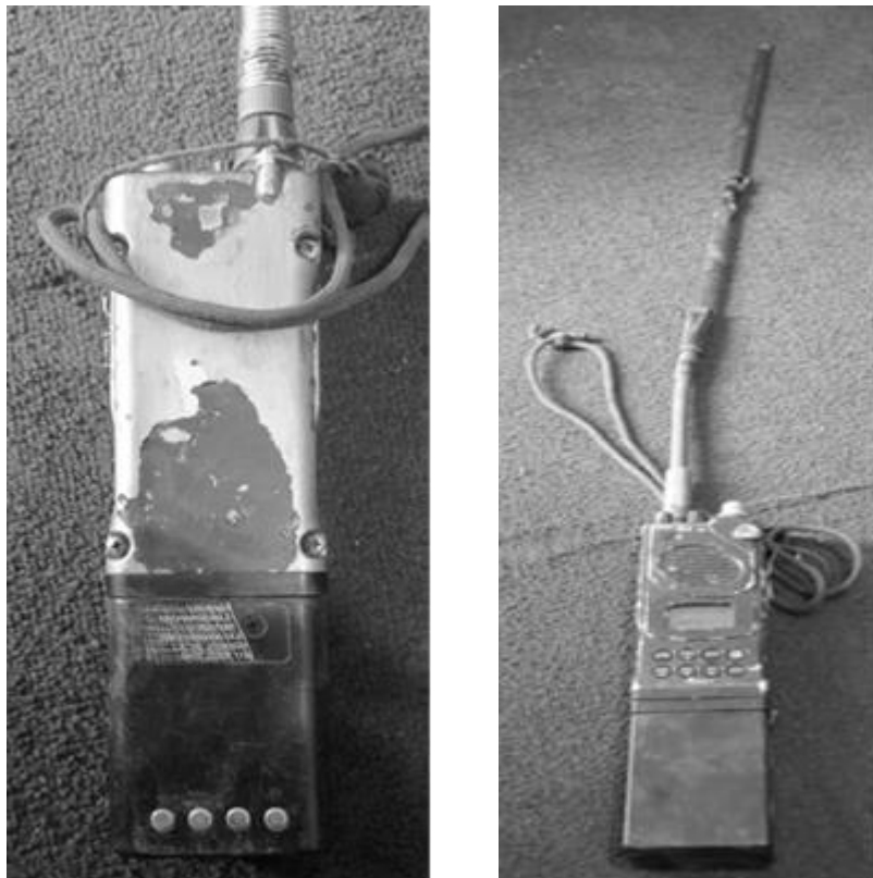
Tadiran RT-7106 (PRC-710) tactical VHF/FM radio transceiver. The attached TEL-718B battery unit is visible at the base. Confidential source
