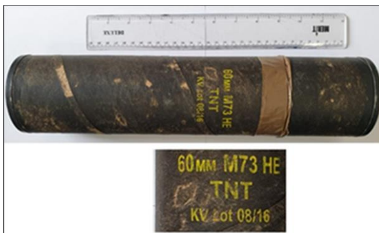
Figure 2: Casing of 60mm mortar round
