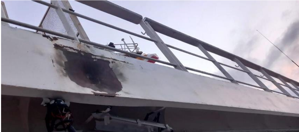
Figure 4: RPG's impact on the vessel.
